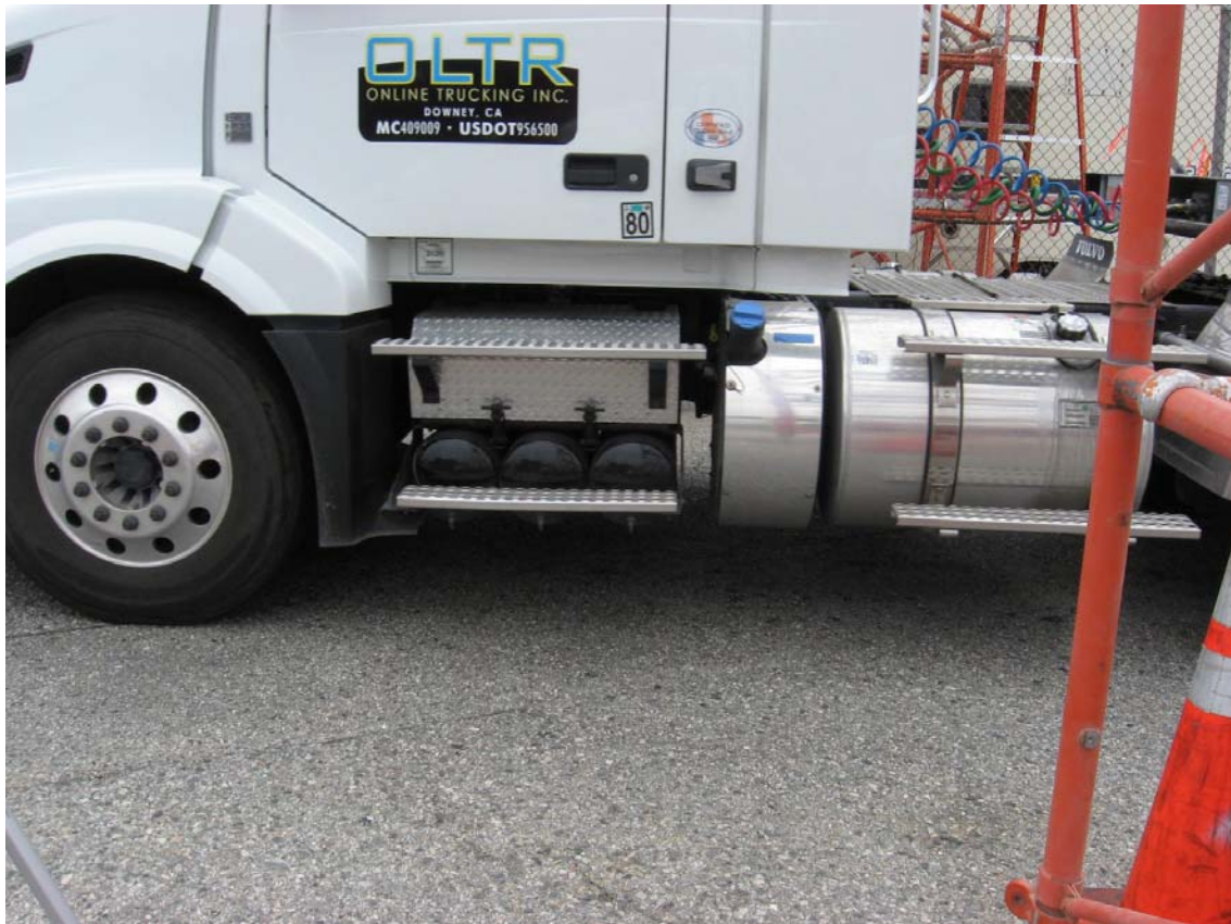
Figure 7. Driver side image of a truck leaving our port location with the urea tank clearly visible.
