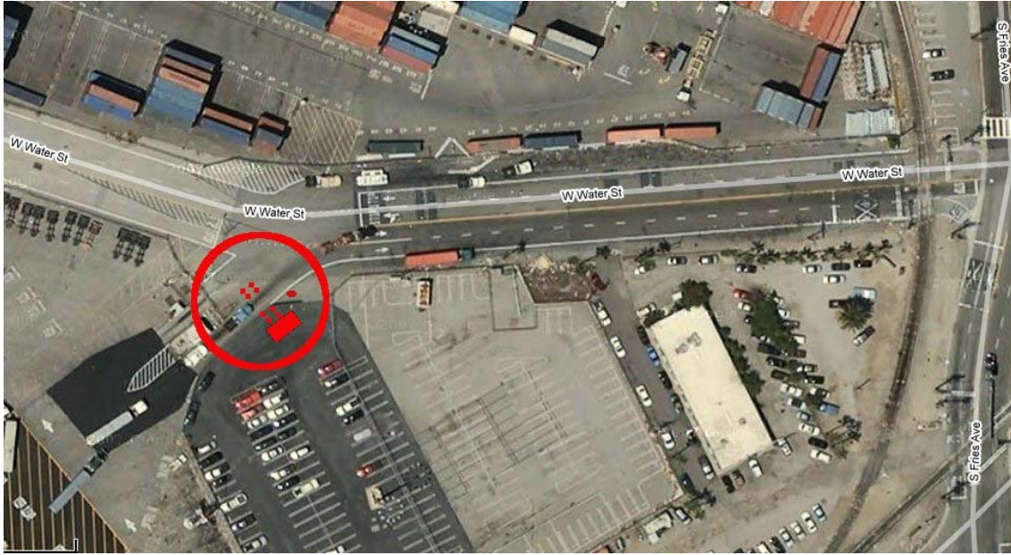
Figure 4. A satellite photo of the Port of Los Angeles Water St. exit. The measurement location is circled in the lower left with approximate locations of the scaffolding, support vehicle and camera.
