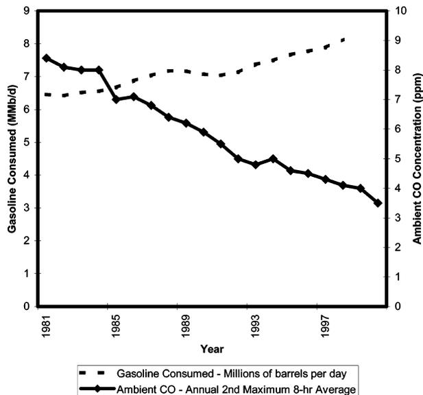
FIGURE 1. Opposite trends in gasoline consumption and CO ambient concentration. The decreasing plot shows EPA reported data on second maximum measured carbon monoxide concentrations in the air of the United States (6), while gasoline consumption by motor vehicles has been increasing (5).
