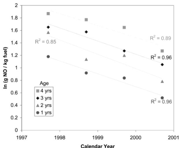
FIGURE 5. The NO data from four measurement campaigns in Chicago. As a reference, the tier 0 federal 50 000 mile standard of 1.0 g/mi emissions as ( $\text{NO}_2$ ) for light duty vehicles transforms to 5.4 gNO/kg fuel, assuming a fuel economy of 23 mpg. This standard would appear at 1.7 on the log scale in the figure. The 0.4 g/mi Tier 1 standard would be 0.74 on the log scale.
