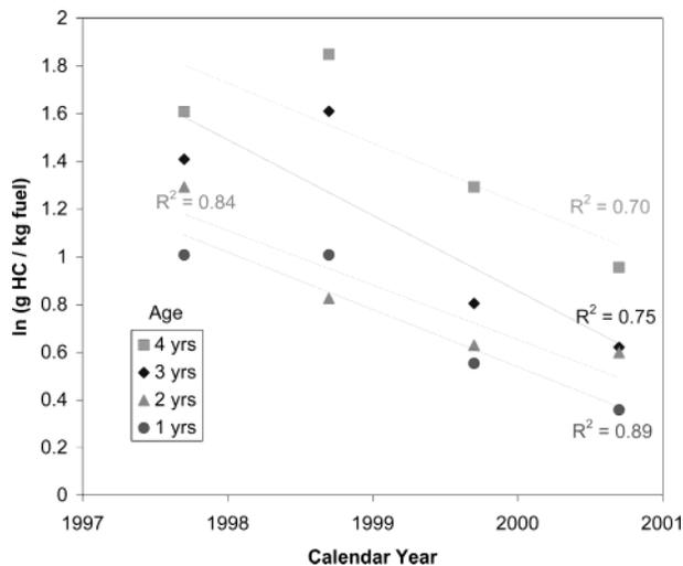
FIGURE 4. The HC data from four measurement campaigns in Chicago. As a reference, the tier 0 and tier 1 federal 50 000 mile standard of 0.41 g/mi HC emissions for light duty vehicles transforms to 3.4 g HC/kg fuel, assuming a fuel economy of 23 mpg. This standard would appear at 1.2 on the log scale in the figure.
