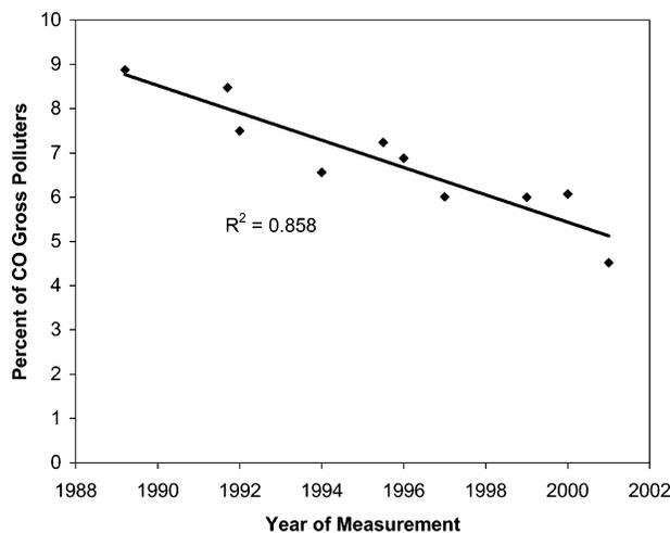
FIGURE 2. Decrease in fraction of CO gross polluters during measurements in Denver from 1989 to 2001. Gross polluters are defined as the percentage of the total measured fleet responsible for 50% of total measured CO emissions.
