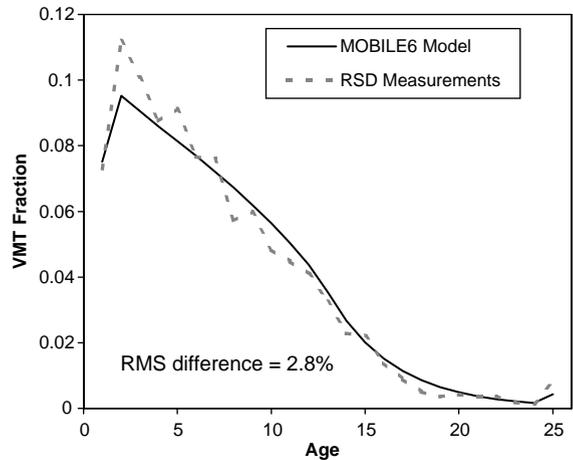
Fig. 1. Relative travel fractions of passenger cars as a function of age. Solid line is the MOBILE6 national average default values. The broken line is the measurement frequency in remote sensing.
