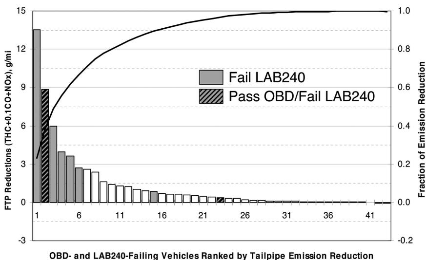
**Figure 1.** Cumulative net exhaust emission reductions, and fraction of emission reductions (solid line) for the 43 on-board diagnostic equipment (OBD)/MIL and LAB240-failing vehicles, in rank-order from largest to least emission reductions. The gray bars are vehicles that failed the LAB240; the cross-hatched bars are the two OBD error-of-omission vehicles.
