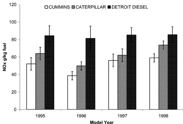
**FIGURE 3.** NO<sub>x</sub> emissions for the three most represented engine manufacturers from this study during the model years preceding the 1998 consent decrees. Uncertainties are the standard errors of the mean.
