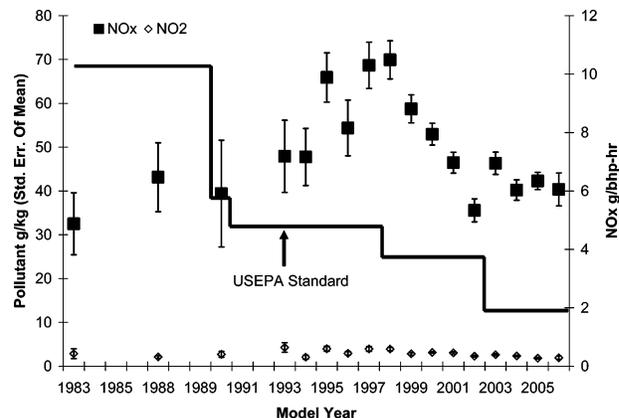
**FIGURE 2. Mean NO<sub>x</sub> and NO<sub>2</sub> emissions plotted versus VIN model year. The solid line represents the new engine certification standards in g/bhp-h. The two y-axes have been plotted together assuming 0.15 kg of fuel consumed per bhp-h for all model years. The uncertainties are the standard errors of the mean.**
