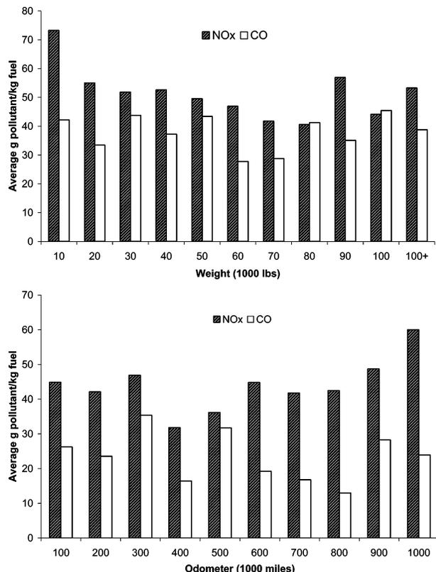
**FIGURE 1. Plot of NO<sub>x</sub> and CO emissions versus GVW as measured by the weigh station scales (top) and odometer mileage as reported by the truck driver (bottom).**
