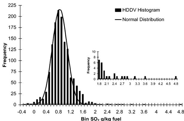
**FIGURE 4.** The histogram of combined SO<sub>2</sub> emissions from the two measured sites. The solid line represents the least-squares fit normal distribution associated with a mean of 0.84 g/kg SO<sub>2</sub>. The insert contains the 27 measurements with SO<sub>2</sub> values greater than the 99.9% confidence interval.
