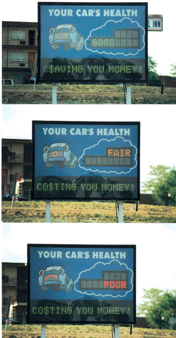
FIGURE 2. Photographs of the Smart Sign as deployed. The GOOD message and car smile are green led's, the FAIR message and car ooh are amber led's, and the POOR message and car frown are red led's. The bottom message is display in green led's for both messages.
