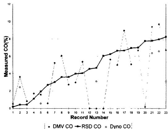
Fig. 3. Comparison of all three measurement techniques by individual vehicles for one day at the Hadland Park roadside pullover site in Las Vegas. See Fig. 2 caption for details.
