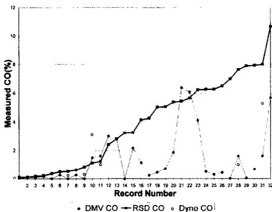
Fig. 2. Comparison of all three measurement techniques by individual vehicles for one day at the Kietzke Lane roadside pullover site in Reno. Data are rank-ordered by the DU RSD CO (%). Gross-polluter cutoff was 4.0% CO. Measurements are coded as follows: RSD CO (DU RSD %CO), DMV CO (Average of the DMV high and low idle speed %CO) and Dyno CO (US EPA IM240%CO).
