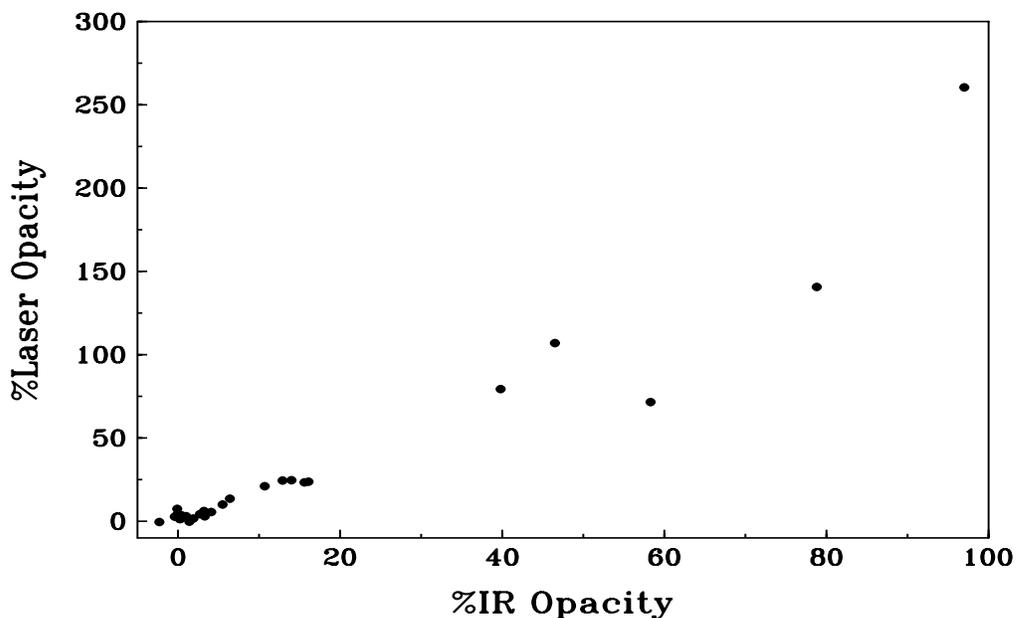
**Figure 5.** A correlation graph using data collected in our parking lot on March 7, 2001 with the Ford F250 truck. This data has been post processed using improved software which allowed the collection of more opaque plumes.
