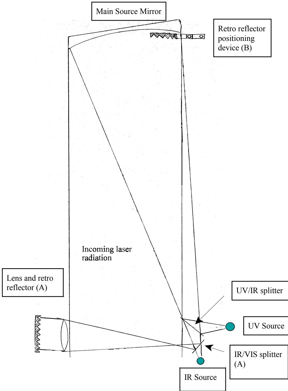
**Figure 2.** Schematic of two source (final design used configuration B) configurations tried to collimate the laser light with the current IR/UV sources. Common elements are not lettered.
