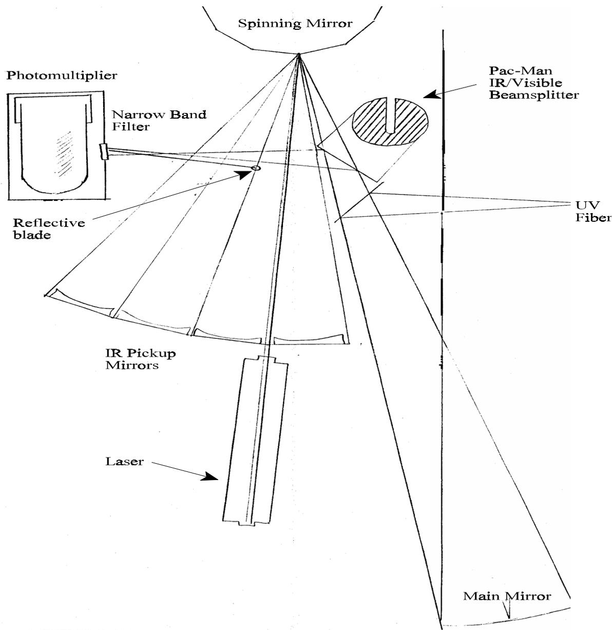
**Figure 3.** Detector system showing the laser beam striking the spinning mirror, exiting via the slit in the Pac-Man and returning to the Pac-Man, thence to be reflected to the PMT. The reference signal is provided by the small reflective blade.
