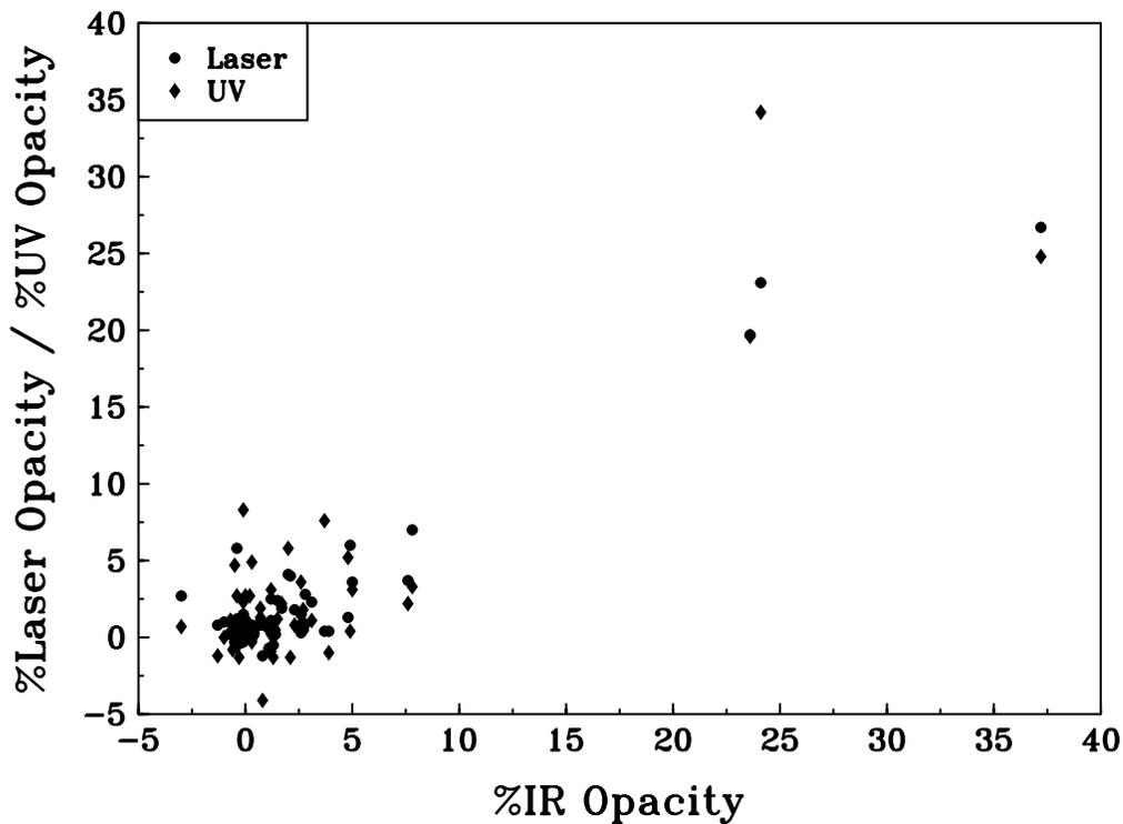
**Figure 4.** Correlation graph between the IR, UV and laser opacity measurements collected in the parking lot on February 21, 2001.
