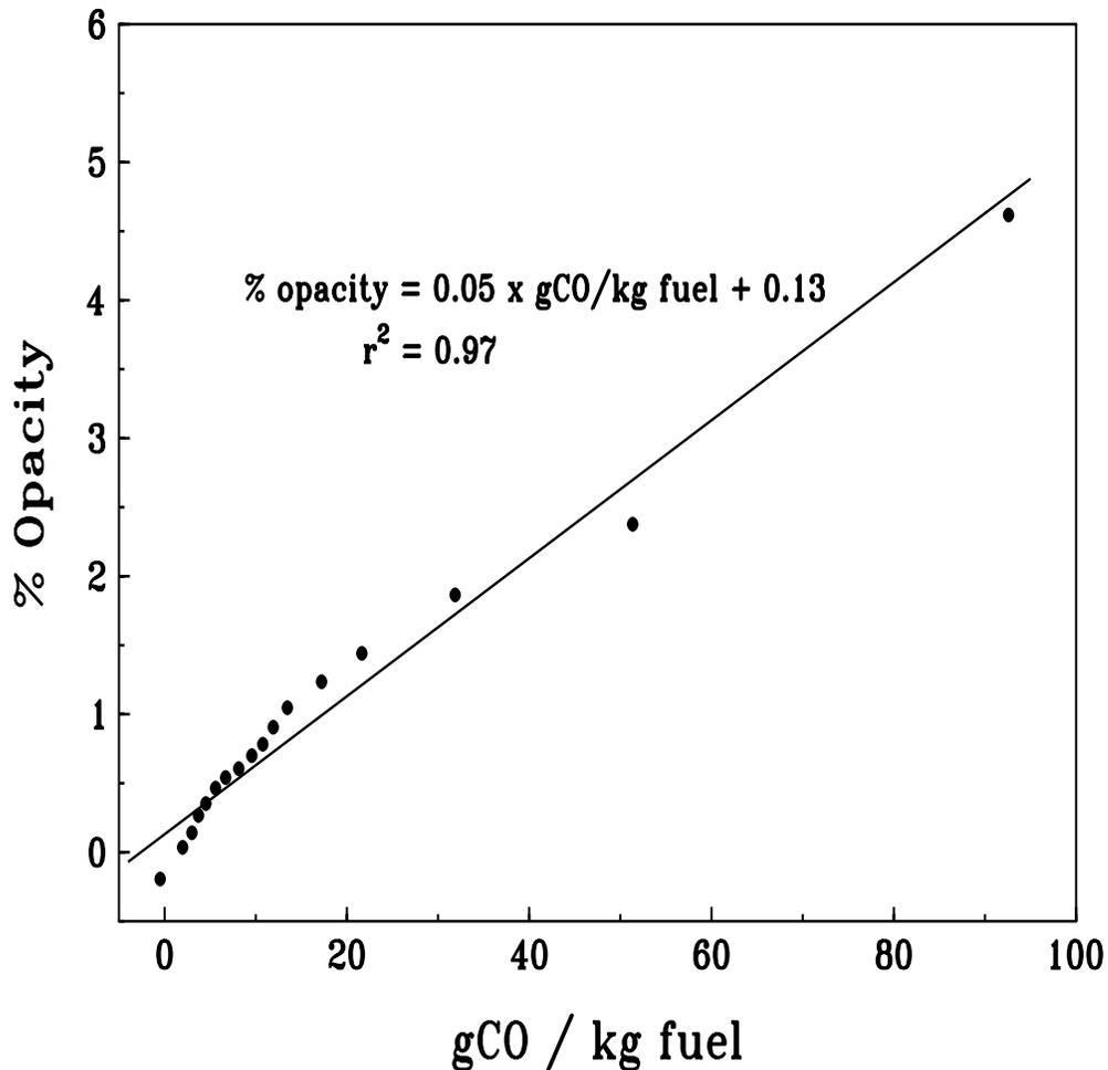
**Figure 1.** A correlation of the average % opacity and g CO/kg fuel of heavy-duty diesel trucks binned by opacity in the Austin-San Marcos Texas area.  $r^2 = 0.97$ .
